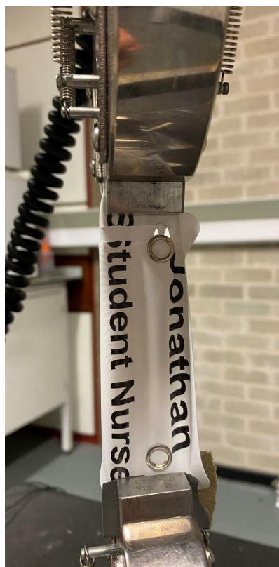
Figure 14: Failure point during tensile strength test.
