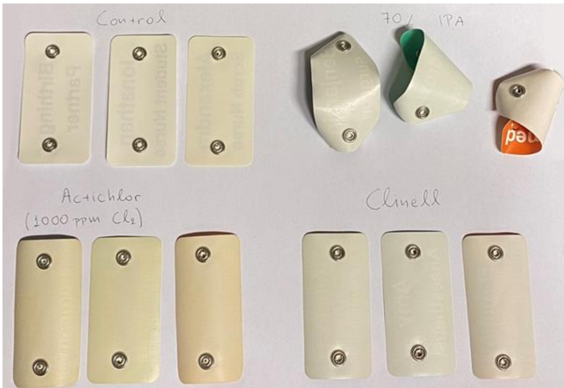
Figure 10: Back side of the polyester badges, post the chemical degradation experiment.
