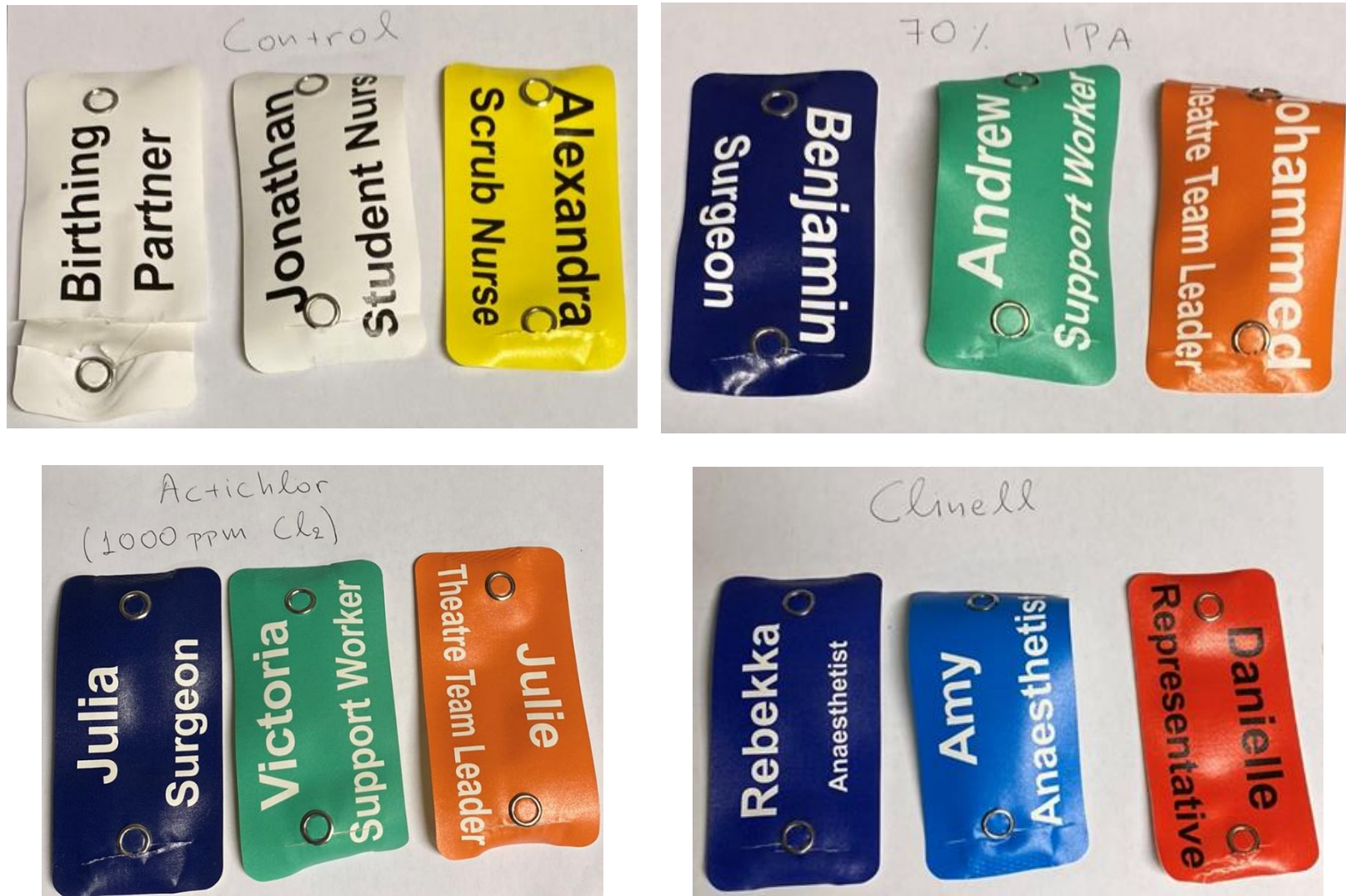
Figure 15: Front side of the polyester badges, post the tensile strength tests.
