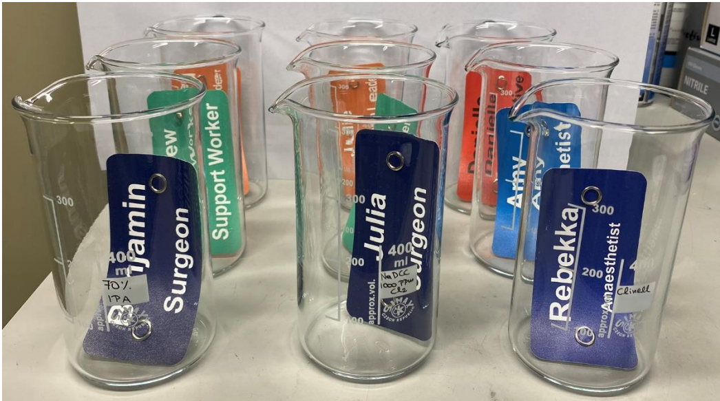
Figure 2: 70% IPA, Actichlor and Clinell test groups, prior to the chemical degradation experiment.
